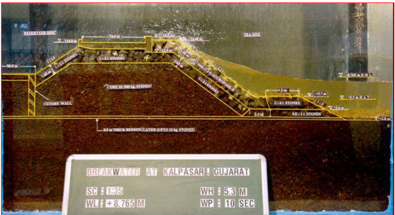
Photo-21 : Wave action on the armour of breakwater cross-section at +2.0 m bed level during breaking wave height (Hs) of 5.3 m at Design Water Level (DWL) of +8.765 m
