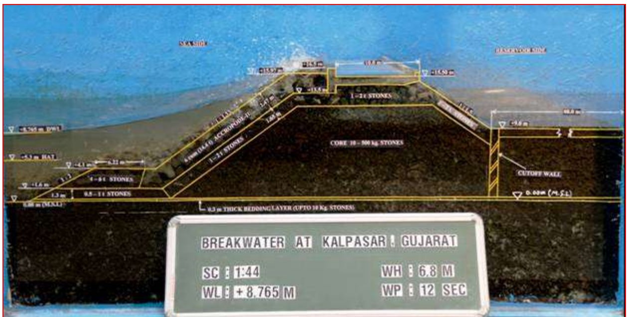
Photo-19 : Wave action on the armour of breakwater cross-section at 0.0 m bed level during breaking wave height ( H_s ) of 6.8 m at Design Water Level (DWL) of +8.765 m
