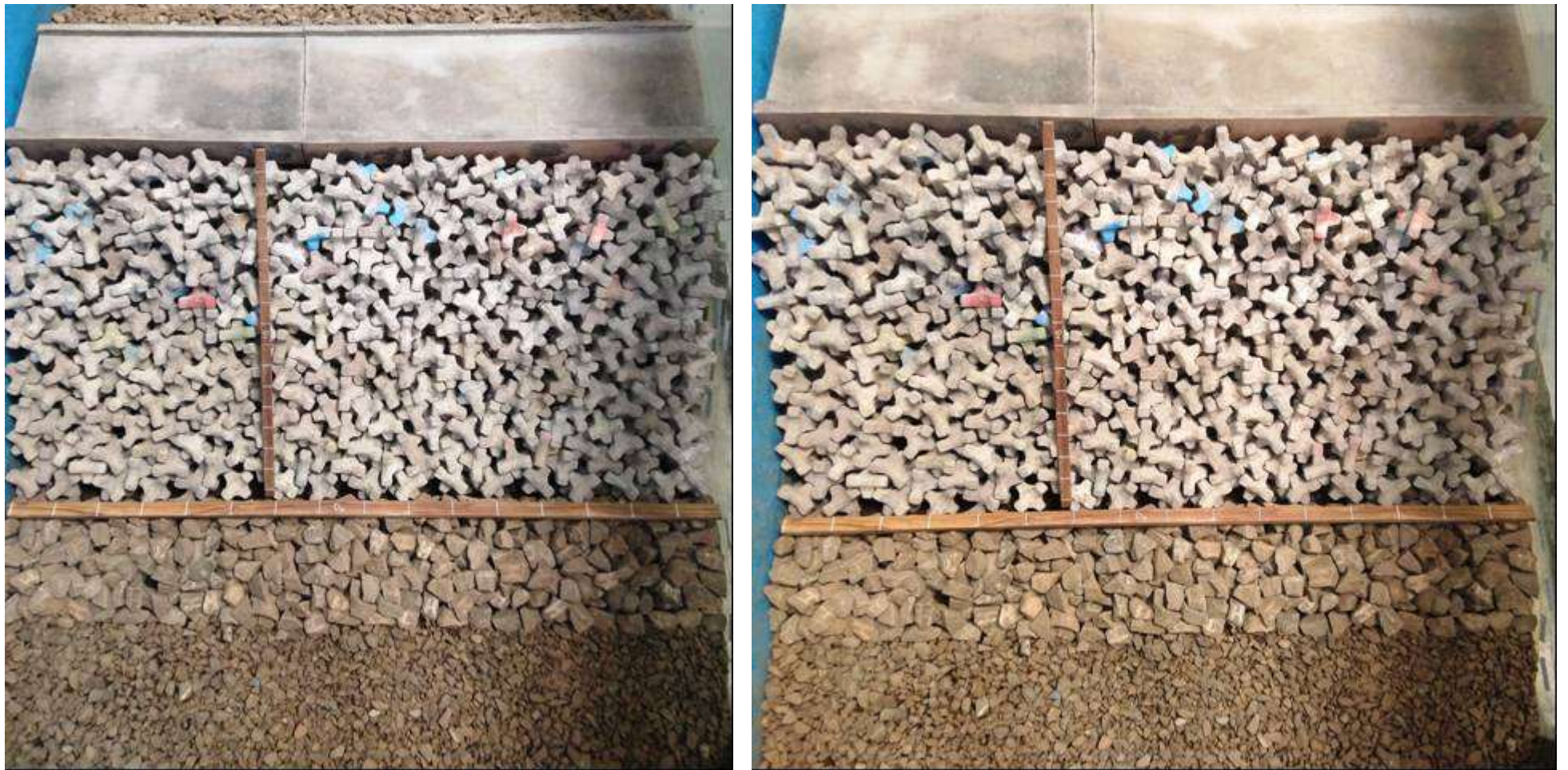
Photo-18 : Placement of Accropode™ II model units in the wave flume at 0.0 m bed level
