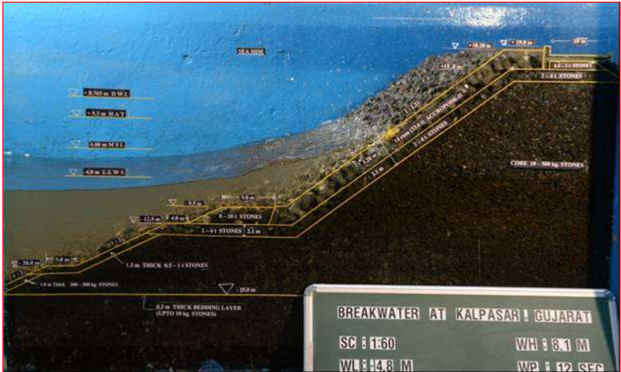
Photo-16 : Wave action on the armour of breakwater cross-section at -25.0 m bed level during significant wave height ( H_s ) of 8.1 m at Lowest Low Water Level (LLWL) of -4.8 m
