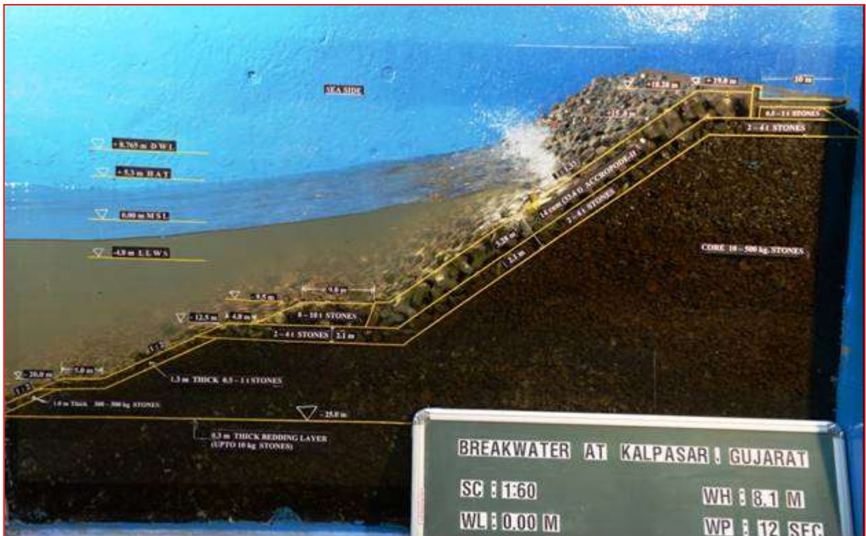
Photo-14 : Wave action on the armour of breakwater cross-section at -25.0 m bed level during significant wave height ( H_s ) of 8.1 m at Mean Sea Level (MSL) Level of 0.0 m
