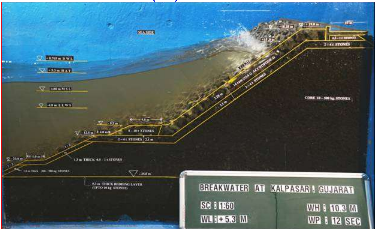
Photo-12 : Wave action on the armour of breakwater cross-section at -25.0 m bed level during significant wave height ( H_s ) of 8.1 m at Highest Astronomical Tide (HAT) Level of +5.3 m
