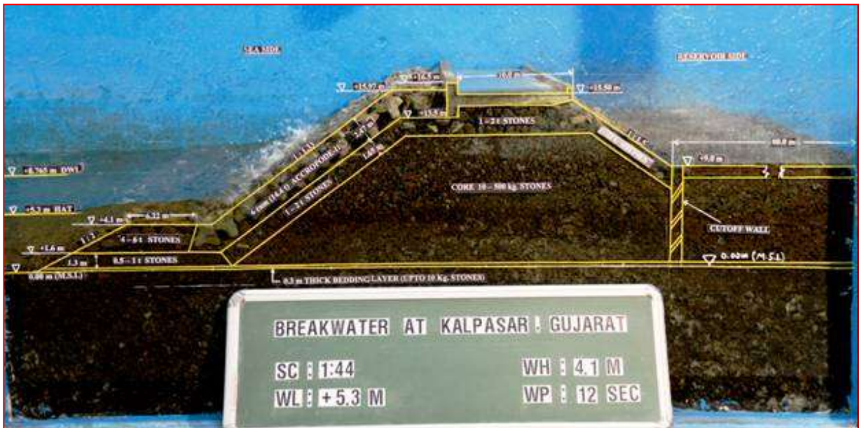
Photo-20 : Wave action on the armour of breakwater cross-section at 0.0 m bed Level during significant wave height (Hs) of 4.1 m at Highest Astronomical Tide (HAT) Level of +5.3 m
