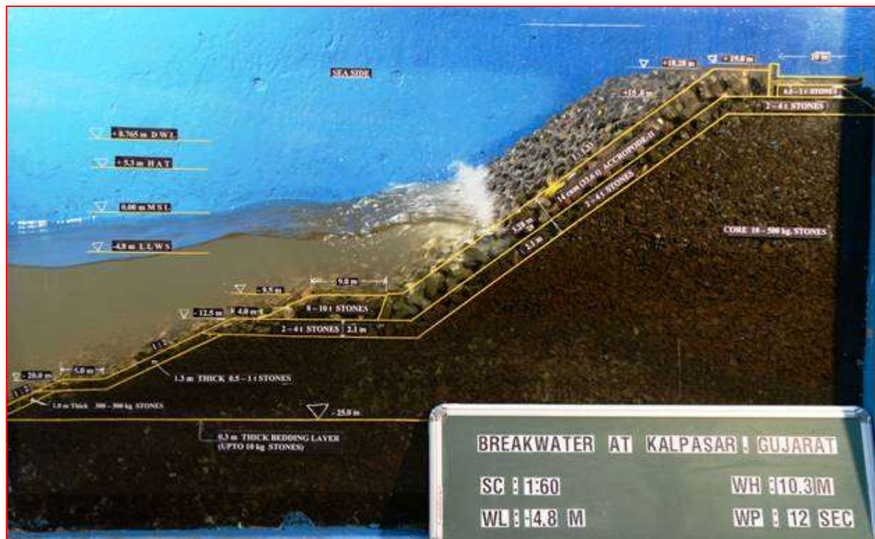
Photo-17 : Wave action on the armour of breakwater cross-section at -25.0 m bed level during maximum breaking wave height ( H_{1/10} ) of 10.3 m at Lowest Low Water Level (LLWL) of -4.8 m
