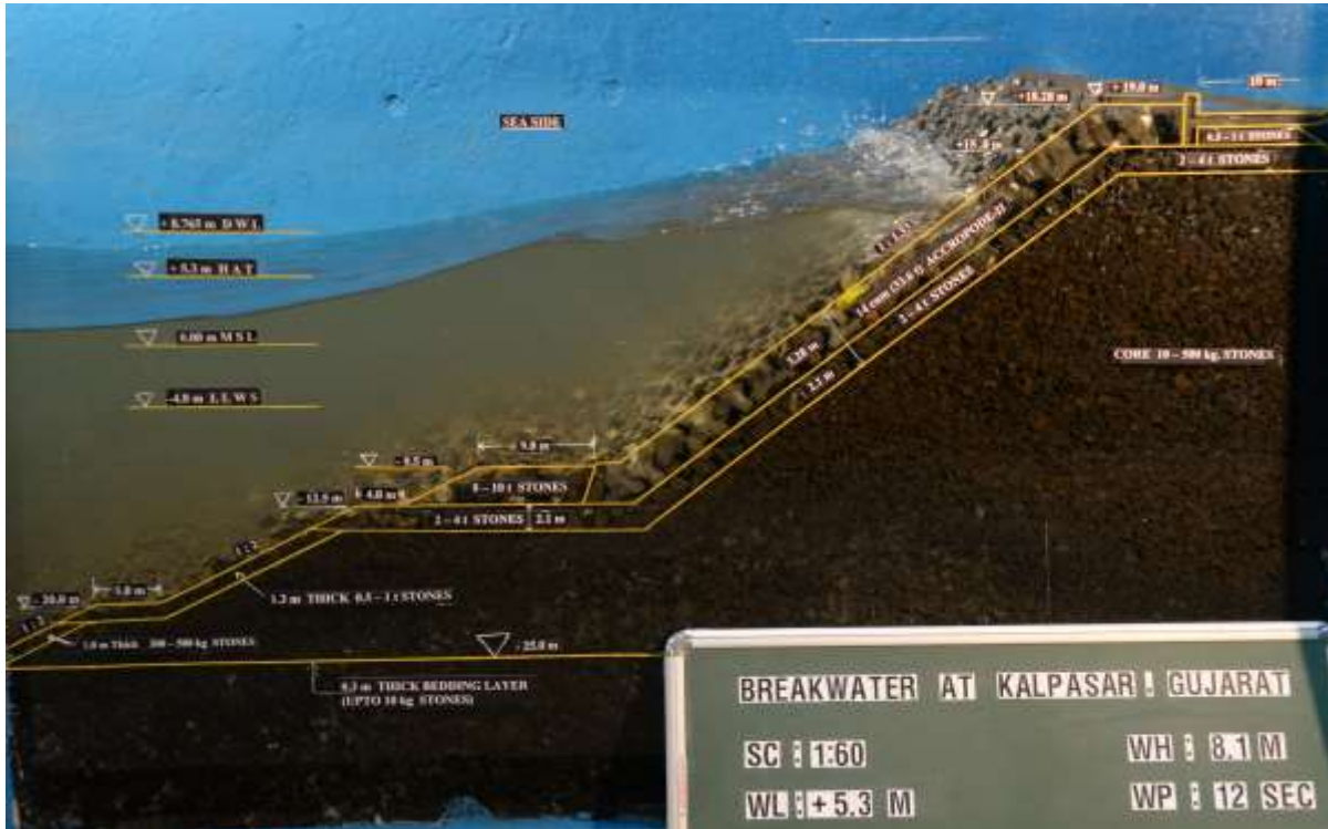
Photo-12 : Wave action on the armour of breakwater cross-section at -25.0 m bed level during significant wave height ( H_s ) of 8.1 m at Highest Astronomical Tide (HAT) Level of +5.3 m
