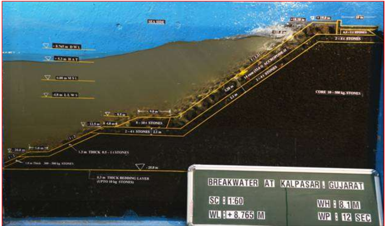
Photo-10 : Wave action on the armour of breakwater cross-section at -25.0 m bed Level during significant wave height ( H_s ) of 8.1 m at Design Water Level (DWL) of +8.765 m
