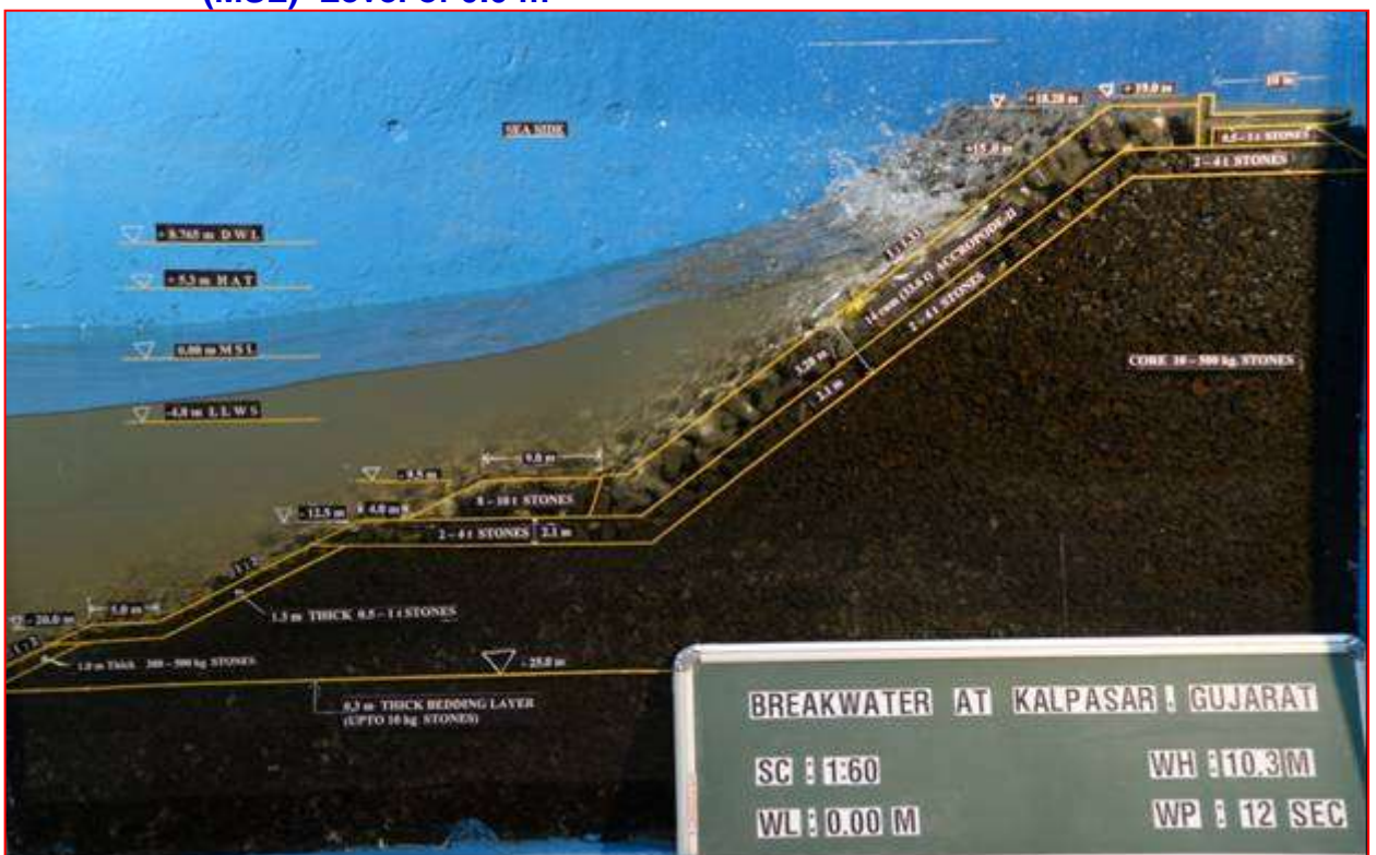
Photo-15 : Wave action on the armour of breakwater cross-section at -25.0 m bed level during maximum breaking wave height ( H_{1/10} ) of 10.3 m at Mean Sea Level (MSL) of 0.0 m
