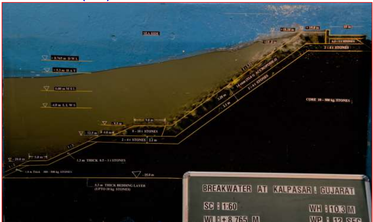
Photo-10 : Wave action on the armour of breakwater cross-section at -25.0 m bed Level during significant wave height ( H_s ) of 8.1 m at Design Water Level (DWL) of +8.765 m
