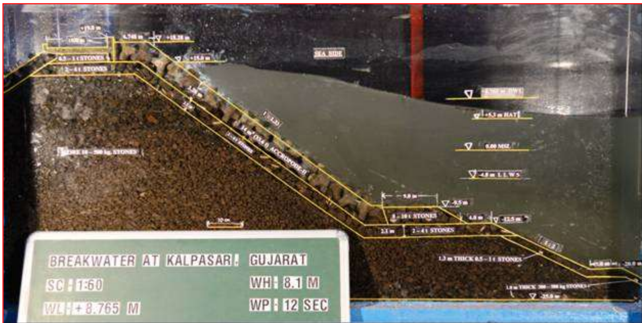
Photo-6 : Wave action on the armour of breakwater cross-section at -25.0 m bed level during significant wave height ( H_s ) of 8.1 m at Design Water Level (DWL) of +8.765 m
