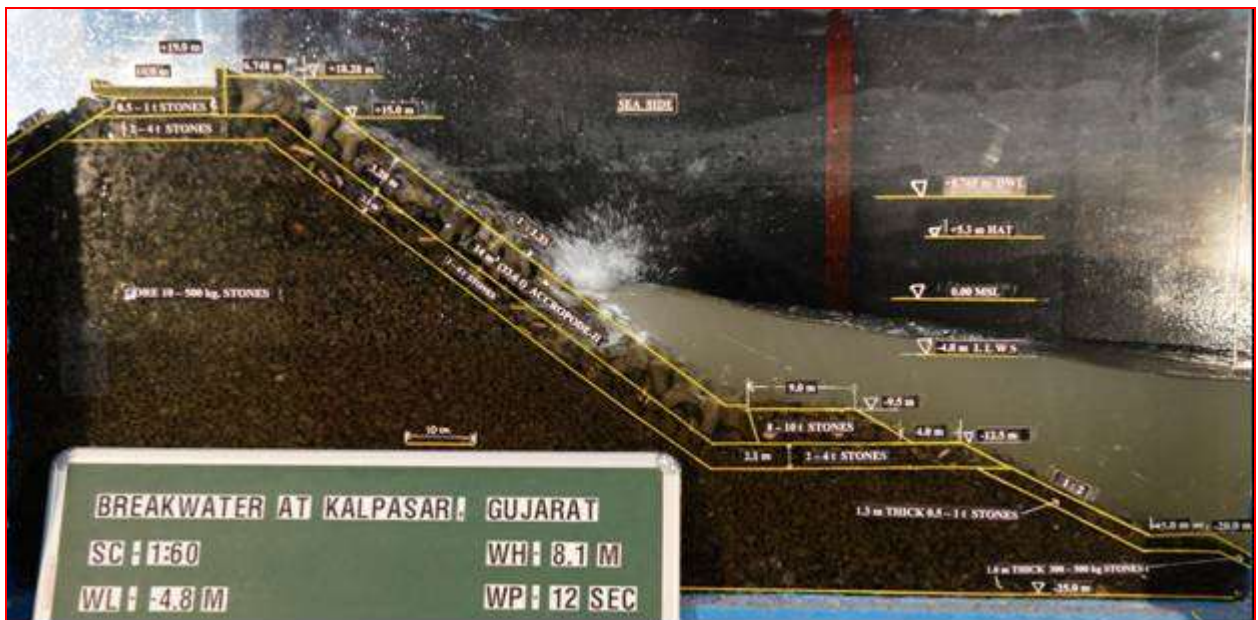
Photo-9 : Wave action on the armour of breakwater cross-section at -25.0 m bed level during significant wave height ( H_s ) of 8.1 m at Lowest Low Water Level (LLWL) of -4.8 m
