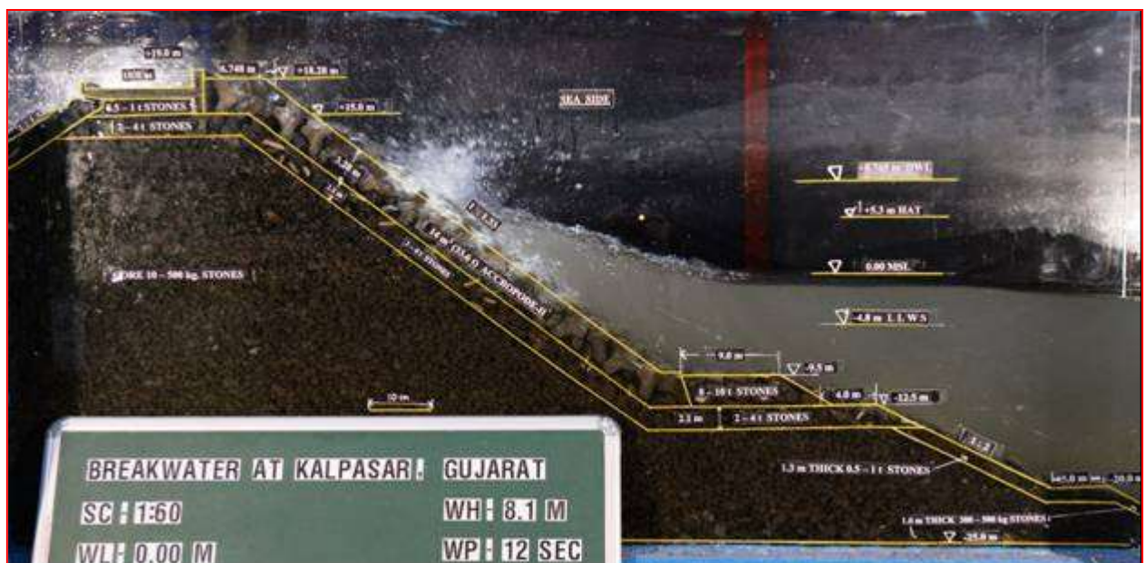
Photo-8 : Wave action on the armour of breakwater cross-section at -25.0 m bed level during significant wave height ( H_s ) of 8.1 m at Mean Sea Level (MSL) Level of 0.0 m
